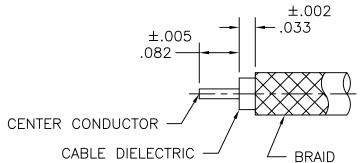
3. PLACE CENTER CONTACT INTO APPROPRIATE LOCATOR/HOLDING TOOL, HEAT CENTER CONTACT AND PUSH OVER CENTER CONDUCTOR OF CABLE UNTIL IT FIRMLY RESTS AGAINST CABLE DIELECTRIC. SOLDER CONTACT IN PLACE.
